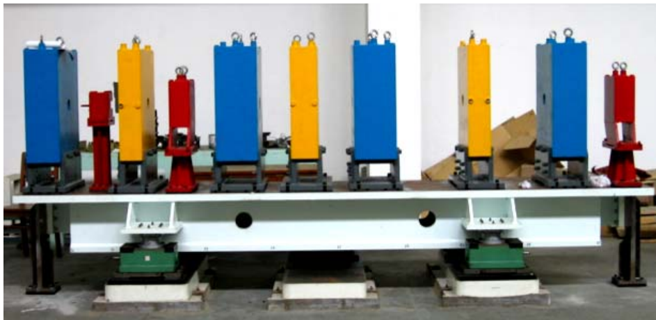
Figure 2: the girder-magnet assembly prototype with damping links assembled to the two ends
