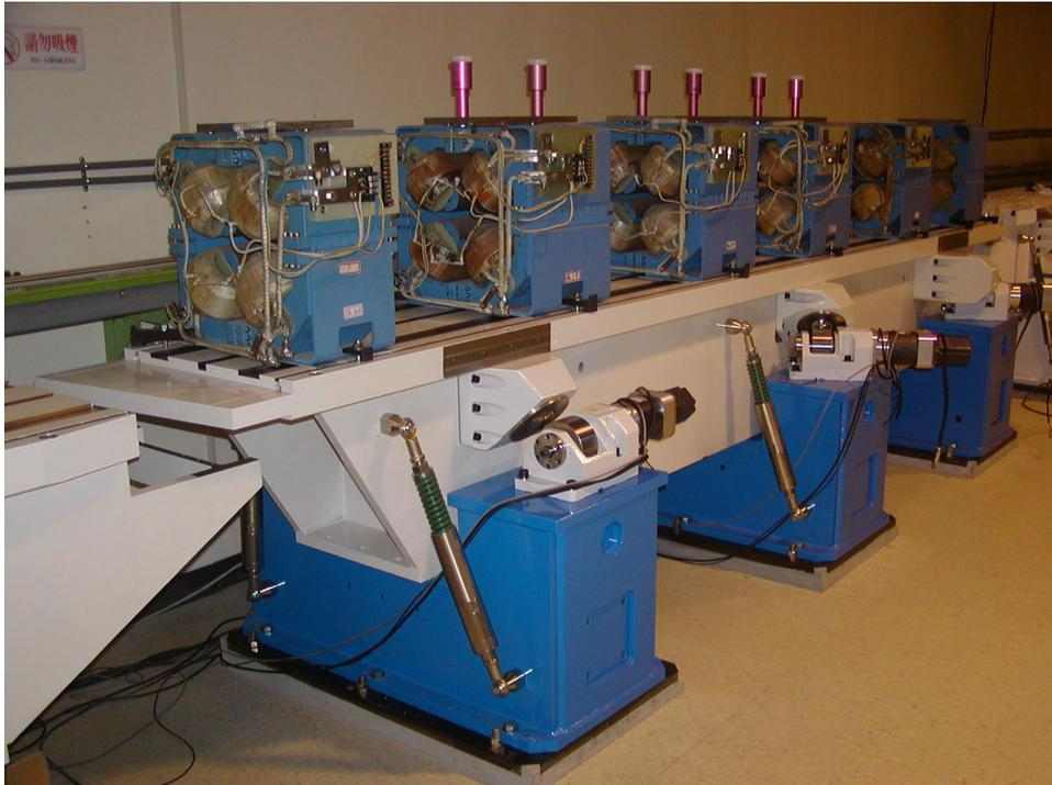
Figure 9: Prototype girder system with quadruples (TLS) for testing
