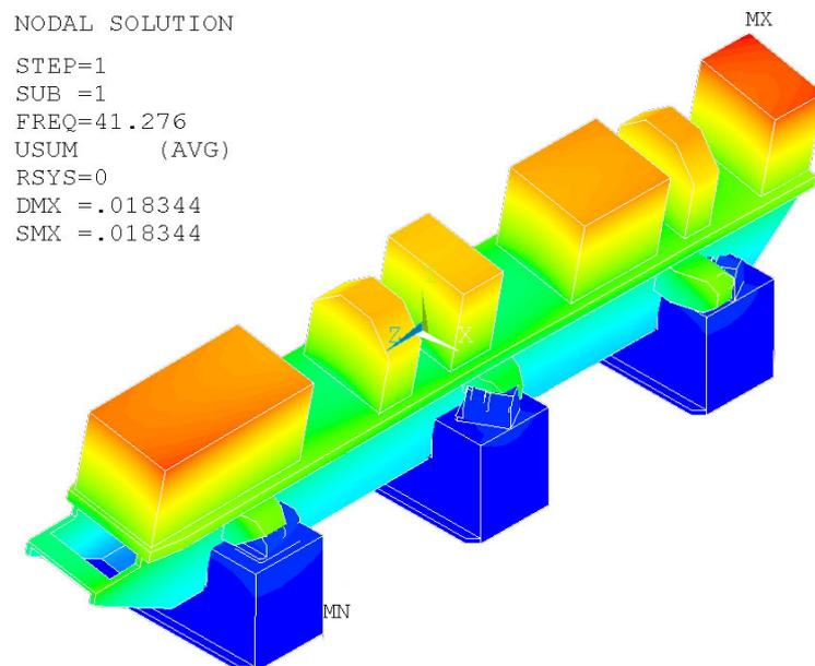
Figure 8: A simple modal analysis by setting the girder and the ball down 10  $\mu$ m and simulating the whole system as one body.
