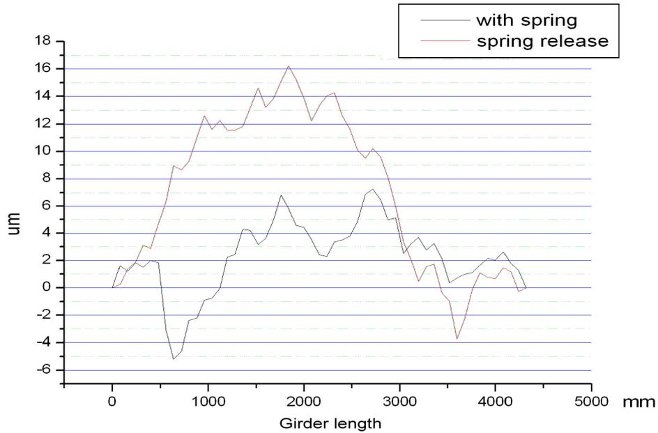
Figure 11: Girder surface flatness measurement by autocollimator after installed
