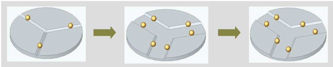
Figure 1: Expand 3-Groove Type kinematic Mounting from 3 balls to 6 balls
