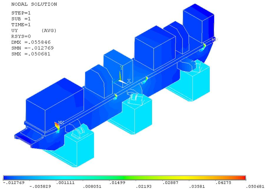
Figure7: With the compensation of assistant springs it is able to keep the girder surface flatness within 5mm from simulation
