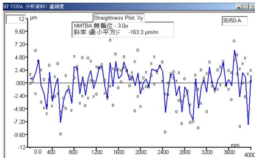
Figure 10: Girder surface flatness measurement by HP 5529A laser at factory.
