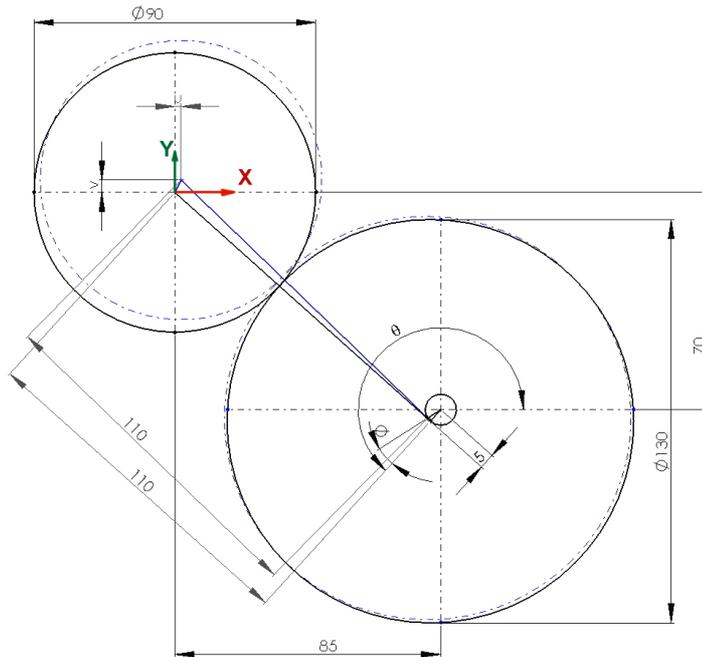
Figure 5: The relations between ball and mover and the coordinate at this system
