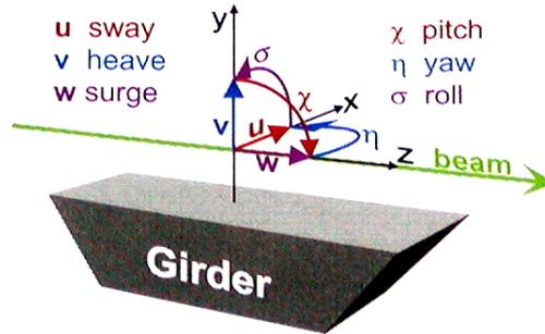
Figure 4: Definition of coordinates of the girder ( This Figure borrowed From [7] )
