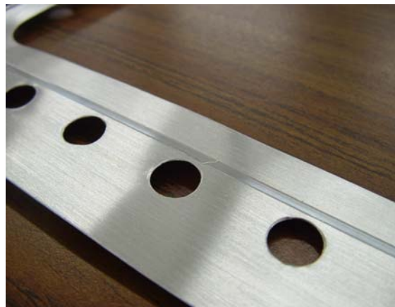
Figure 10. A used AL-gasket on the working bench showing equally apart holes and dented sealing track
