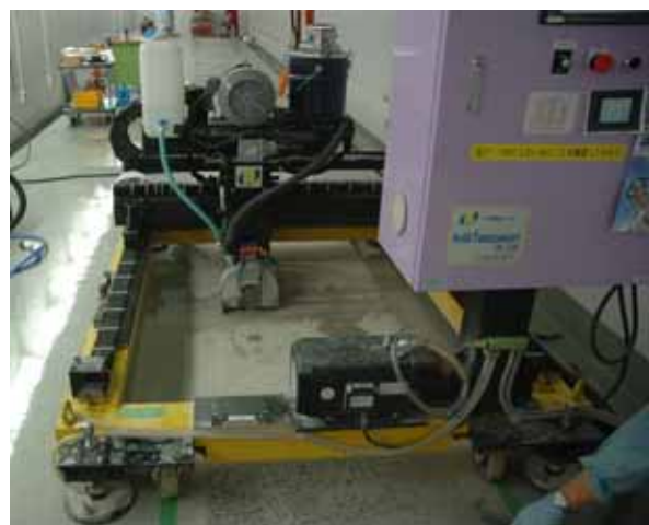
Fig.2 Concrete floor grinding machine.
